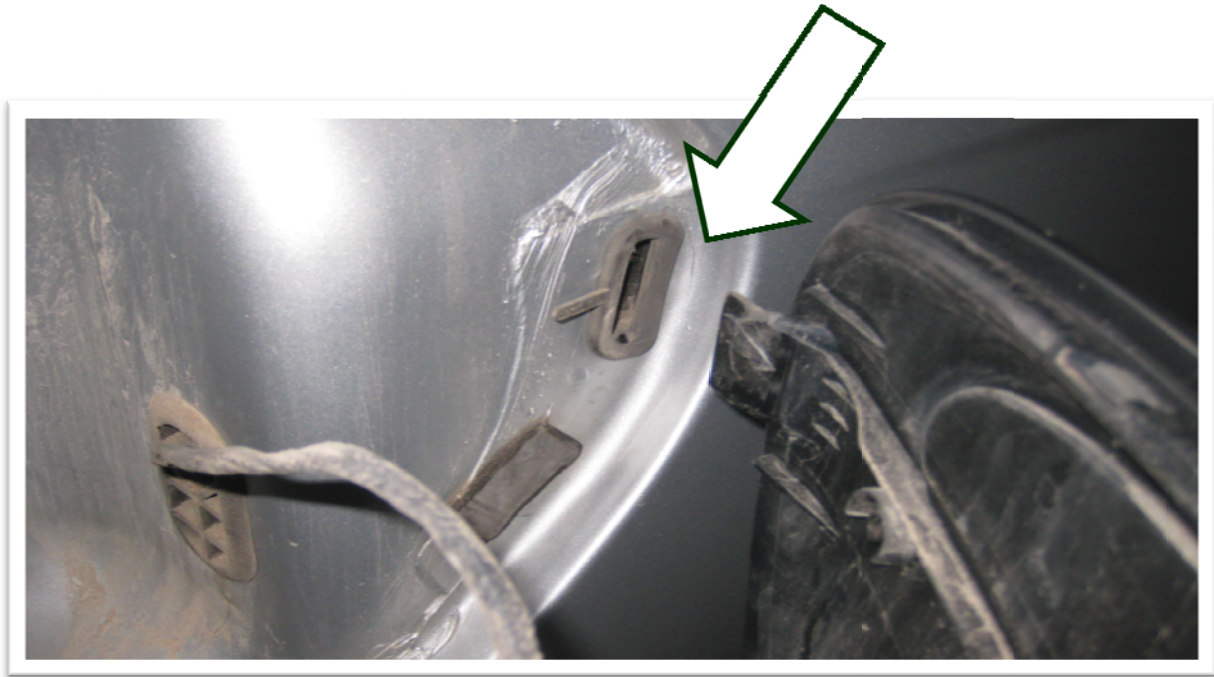
Figure 7. Illustration of a tab being used to locate and retain the front edge of a tail light
